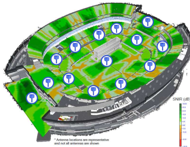
Figure 6: Simulating 5G NR mmWave (28 GHz) at NFL stadium.
